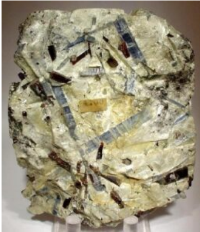
10.6 Porphyroblasts of kyanite (blue) and staurolite (brown) in silvery paragonite; sample from Ticino Canton, Switzerland
