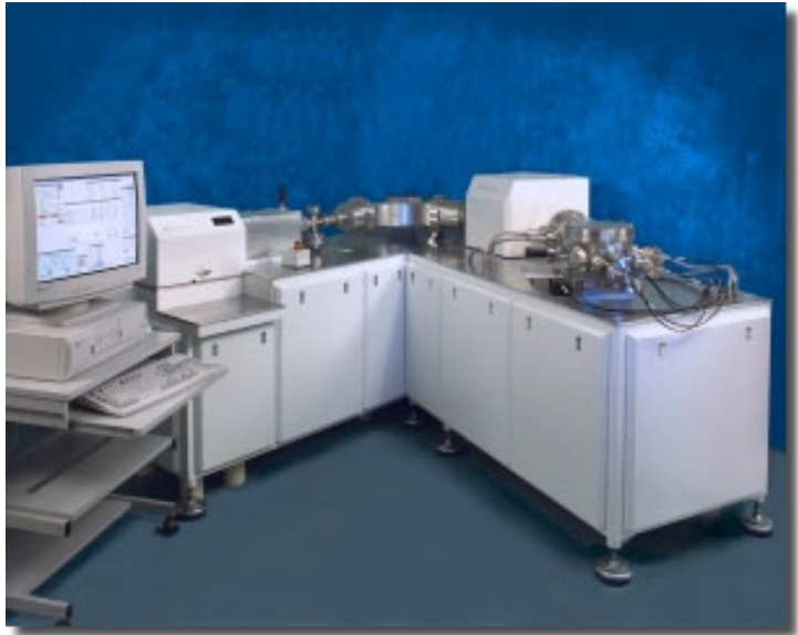
1.8 An inductively coupled plasma mass spectrometry (ICP-MS) at the United States Geological Survey
