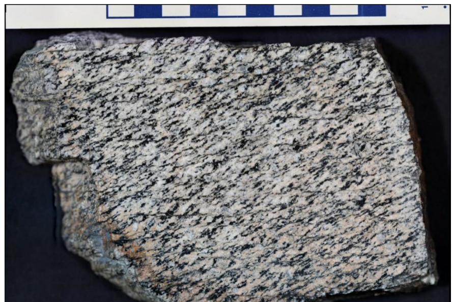
Cross-sectional view of S-C fabric in Rush Creek Granodiorite, near Gem Lake, California.
