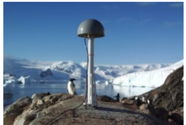
GPS receivers can measure the movement of Earth's landmasses very precisely.
