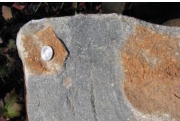
Diabase is a mafic igneous rock found in the Culpeper Basin of Virginia. Note the difference between the rusty weathering rind and the fresh surface, which is dark. Callan Bentley photo.
